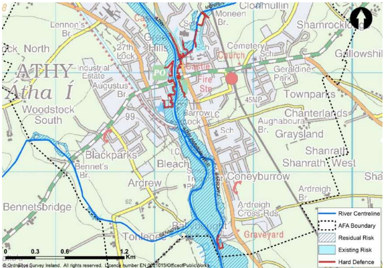
Figure 6-1 Proposed flood relief measures identified in the River Barrow FRMP for Athy
